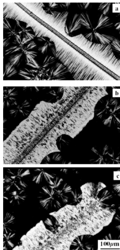
Figure 2. Polarized optical micrographs of iPP fiber/matrix homogeneity composites, which were prepared by introducing the fiber F1 into its single polymer melts at (a) 167, (b) 178, and (c) 185 °C and then cooled to 135 °C for isothermal crystallization.
